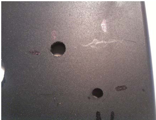
Figure 8-3. Drill holes for the ultrasonic bracket.
