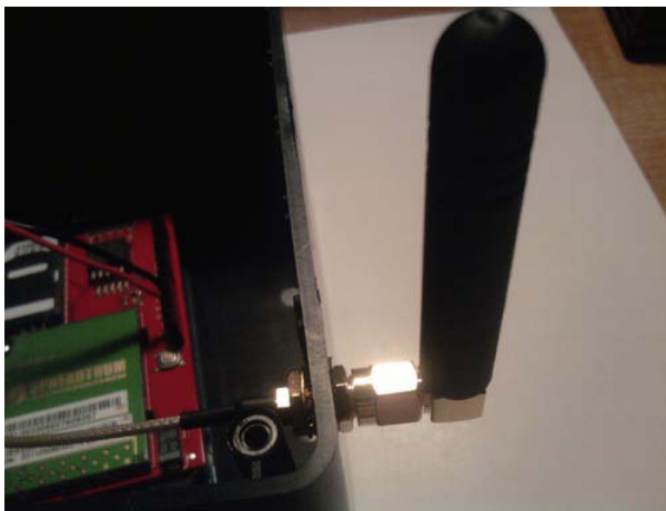
Figure 9-7. Attach duck antenna to SMA connector on Cellular Shield.
