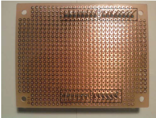
Figure 11-5. Solder on the headers that will connect to the Arduino.
