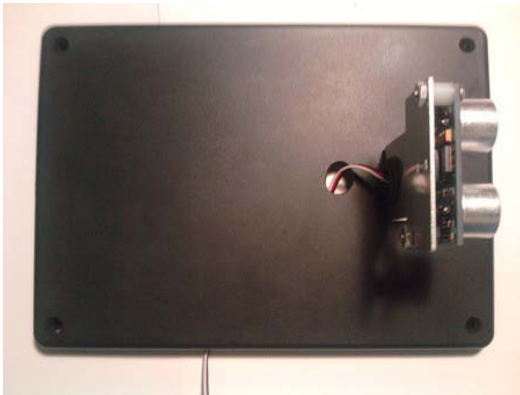
Figure 8-6. Attach ultrasonic sensor to bracket.
