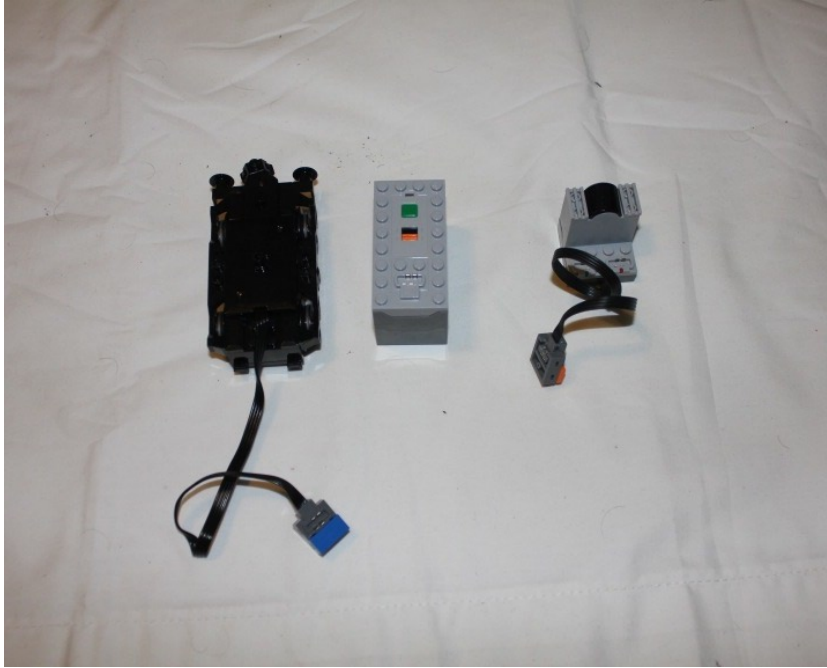
Figure 6-10. The powered wheels, battery box, and IR receiver
